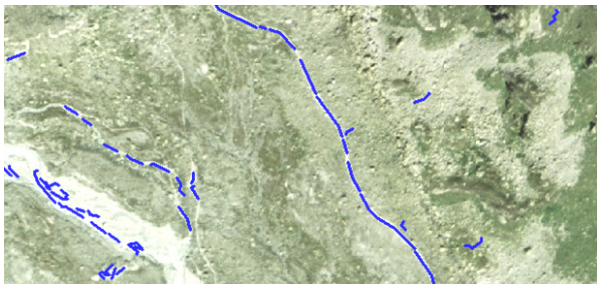
Figure 5. Detail view of walking path extraction result (after vectorisation, "Generalize" and "Line Remove").
